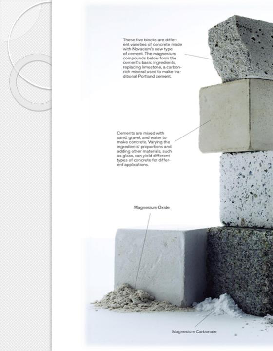
As Novacem's cement hardens, carbon dioxide from the atmosphere is absorbed.
